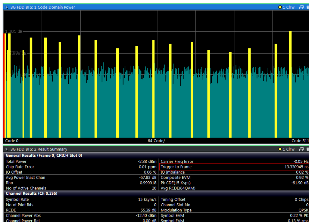
Fig. 8-4: Measurement Example 2: Triggered Measurement of Relative Code Domain Power
